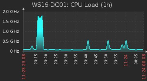
■ CPU usage [avg] last 64 MHz min 55 MHz avg 181.35 MHz m 1.77
